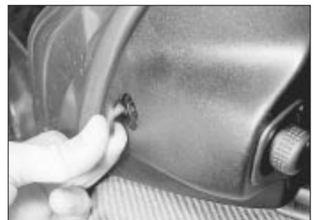
17.12a Prise the securing screw cover from the mirror control panel . . .
