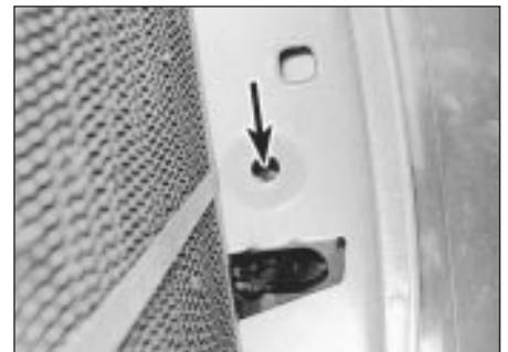
7.9 Access hole (arrowed) below bonnet lock
