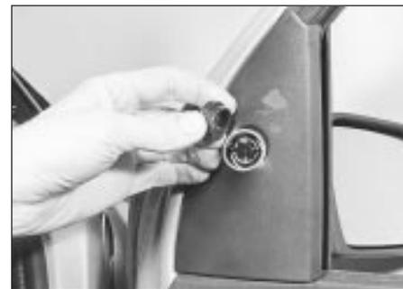
**29.1 Unscrew the bezel from the adjuster knob . . .**
